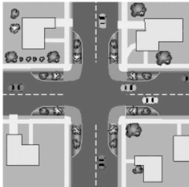
Figure 34 Using Bulbouts for Traffic Calming
